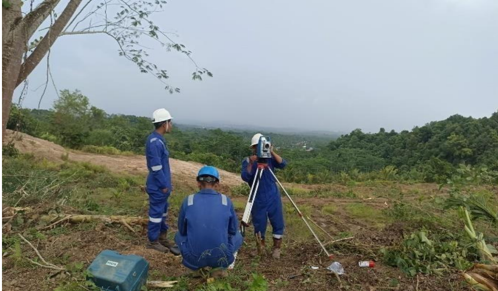
Gambar 10. Pengukuran Stake Out Menggunakan Total Station Spectra Focus
