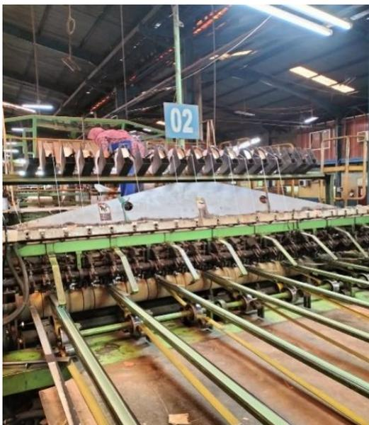
Gambar 9. Mesin core veneer
