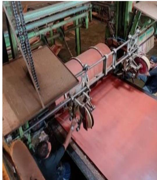
Gambar 6. Mesin *rotary*
