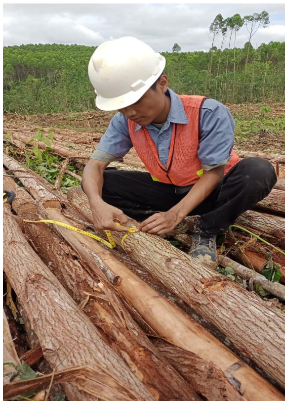
Lampiran 10. Gambar Pengukuran Diameter Log Acacia mangium
